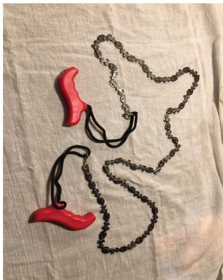
*Manual double sided 53 inch chain saw that weighs around 11 ounces*
